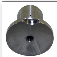
Bottom of reflection target indicating beam direction
