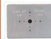
The JIMA resolution chart for testing high resolution micro- and submicrofocus X-ray tubes is available in a new version (RC-02B).
